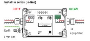
NOTE: For installation in the equipment panel, protectors which are not boxed may be more suitable. If your system requires a protector with a very low resistance, higher current or higher bandwidth use the ESP E or H Series. Unboxed protectors for 3-wire RTD systems are available - as are plug-in protectors for telephone lines and compact Slim Line protectors.
