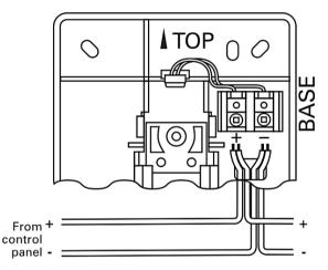
Use both terminal leads for connection. Electrical supervision requires wire run to be broken at each device.
