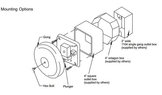
**NOTE:** For octagon outlet box line up the slotted holes to the outlet box mounting holes as shown.
