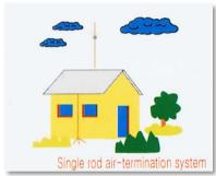
Capturing lightning rod with mast. One or more down conductors. A disconnector on each downconductor to test the resistivity of the structure. A protection element against mechanical forces in the final two meters of the downconductor. An earth electrode for each down conductor. Equipotential bonding of the earth electrodes and general earth termination system.
