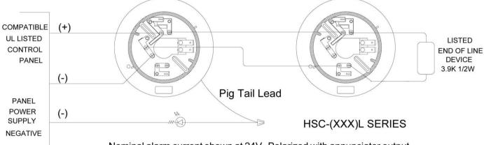
Nominal alarm current shown at 24V. Polarized with annunciator output.
